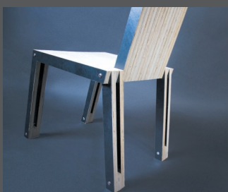
LX3 chair in (20 - 2 cm) marine plywoo slices 40 cm x 62 cm x 76 cm item # 01-07-001 LX3 is one same (boomerang) shape - spin into back, seat and legs; cut from one marine ply-wood sheet, and assembled with bolt and screw (no glue)
